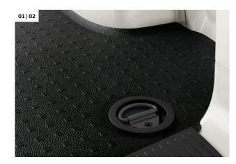
01 Anti-slip, washable rubber floor. Increases safety through an anti-slip surface that extends over the loading sill and the step lighting. | S | H | kombi crew van. | S | H | panel van.
