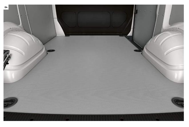
04 Universal floor (for fittings). The ideal preparation for subsequent installation of cabinet systems from various manufacturers<sup>3</sup>. Special adapters<sup>6</sup> in the recesses in the floor covering permit flexible installation of cabinet systems at any time without gluing or drilling. Subsequent removal of the floor leaves only minimum traces. Optional on panel van models. | S | H |
