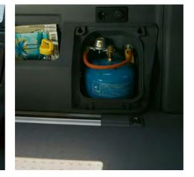
Gas storage compartment. Under the hermetically sealed cover, an optional 1.8 kg Campingaz gas cylinder<sup>1</sup> can be securely attached to straps and connected to the gas hose.
