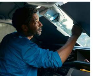
Shades in the cockpit. On California 6.1 Coast and California 6.1 Ocean models, the front windscreen can be blacked out by two roller blinds<sup>1</sup> and the side windows by magnetic curtains.
