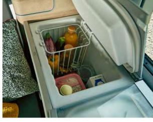
42 litre compressor cool box. The 42 litre chest with clip-on basket, which is easily accessible from above, is cooled by the integrated compressor. Thanks to good insulation and an additional battery, the drinks remain refreshingly cool even during the journey.
