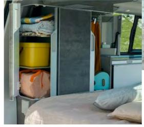
Wardrobe. In the rear section of the California 6.1 Coast and California 6.1 Ocean, is a two-part built-in wardrobe with mirror, clothes rail and lockable safe<sup>2</sup>. Its redesigned doors are easy to open and close.
