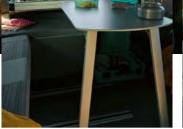
Mini-kitchen with hinged folding table. Stowed safely in the sliding door during the journey, the versatile folding table can be hooked into the guide rail of the folded-out mini-kitchen and placed on two legs if required.
