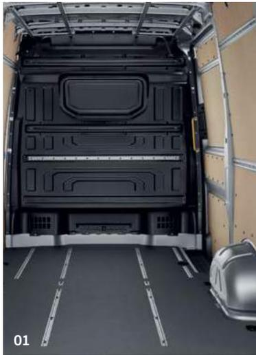
**01 Bulkhead – full-height without window.** A roof compartment above the driver's cabin is available upon request for the high roof variant and is a standard feature with the super-high roof.
