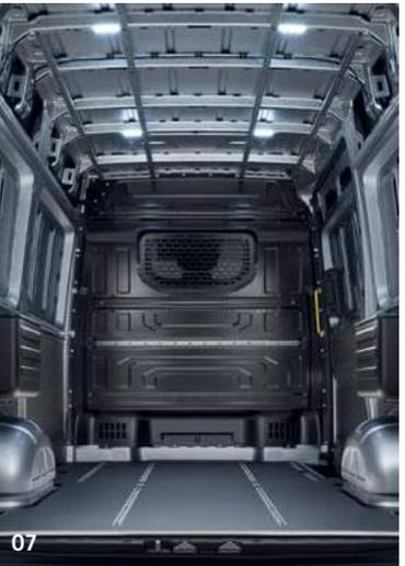
**07 LED load compartment lighting.**<sup>1</sup> Four LEDs integrated into the headlining provide bright and evenly distributed illumination of the load compartment.
