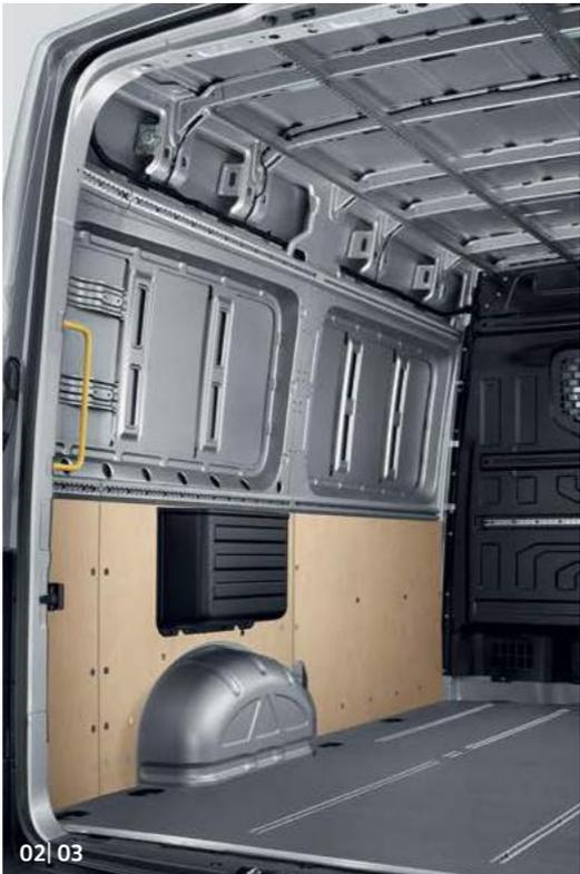
**02 Half-height plywood side lining.**<sup>1</sup> The load compartment cladding made of 5mm thick rigid plywood panels is especially robust. It is fitted from the floor up to the load-lashing rails and is also highly durable.
