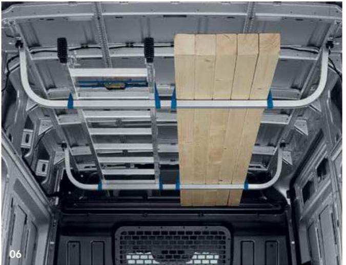
**06 Internal roof rack.**<sup>1</sup> Enables easy transport of long objects. The two rails can be moved within the vehicle and adjusted to the length of the objects. They can also be removed when the roof rack is not needed.
