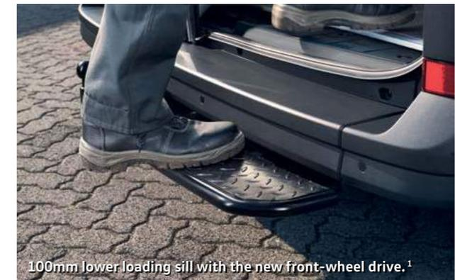
100mm lower loading sill with the new front-wheel drive.<sup>1</sup>
