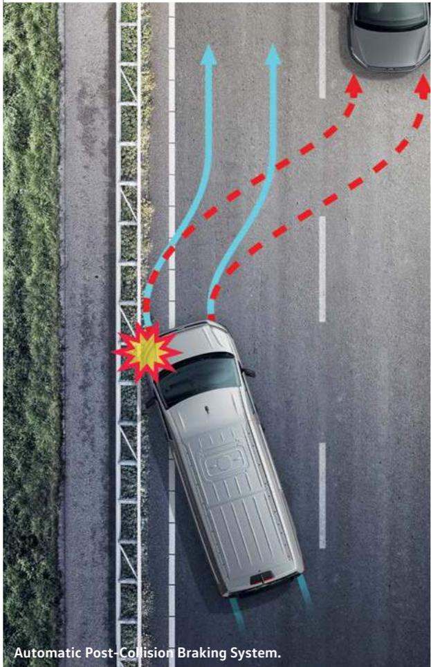
Automatic Post-Collision Braking System.
