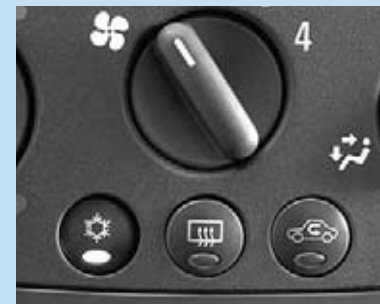
Air conditioning and air recirculation.
